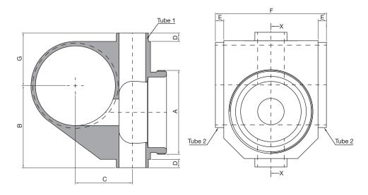
Clean and Aseptic Valves of CAD Product Line have simple and safe design, with their full drainability, without asymptotic seal and dead leg, are offering fast cleanability and sterilization practices. They are designed to fulfil stringent demands of CIP-SIP and Production Cycles on Aseptic Processing.
