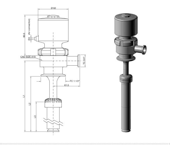
Clean and Aseptic Valves of CAD Product Line have simple and safe design, with their full drainability, without asymptotic seal and dead leg, are offering fast cleanability and sterilization practices. They are designed to fulfil stringent demands of CIP-SIP and Production Cycles on Aseptic Processing.
