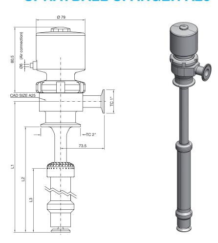
Clean and Aseptic Valves of CAD Product Line have simple and safe design, with their full drainability, without asymptotic seal and dead leg, are offering fast cleanability and sterilization practices. They are designed to fulfil stringent demands of CIP-SIP and Production Cycles on Aseptic Processing.
