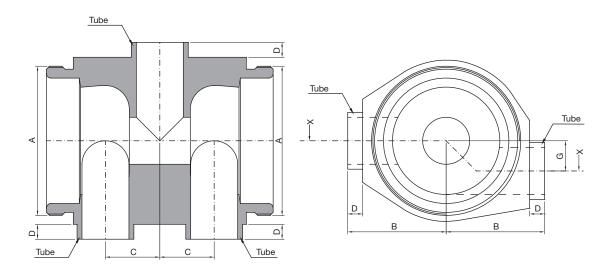
Clean and Aseptic Valves of CAD Product Line have simple and safe design, with their full drainability, without asymptotic seal and dead leg, are offering fast cleanability and sterilization practices. They are designed to fulfil stringent demands of CIP-SIP and Production Cycles on Aseptic Processing.
