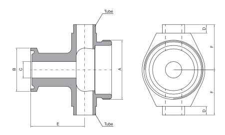
Clean and Aseptic Valves of CAD Product Line have simple and safe design, with their full drainability, without asymptotic seal and dead leg, are offering fast cleanability and sterilization practices. They are designed to fulfil stringent demands of CIP-SIP and Production Cycles on Aseptic Processing.
