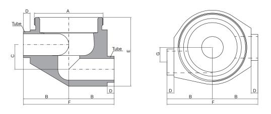
Clean and Aseptic Valves of CAD Product Line have simple and safe design, with their full drainability, without asymptotic seal and dead leg, are offering fast cleanability and sterilization practices. They are designed to fulfil stringent demands of CIP-SIP and Production Cycles on Aseptic Processing.
